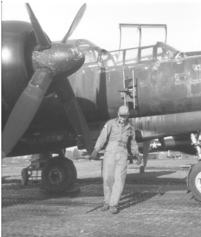
Had to "pull-through" the props on the P-61s big R-2800s every morning, before flight. "Murt" Shields at work.
