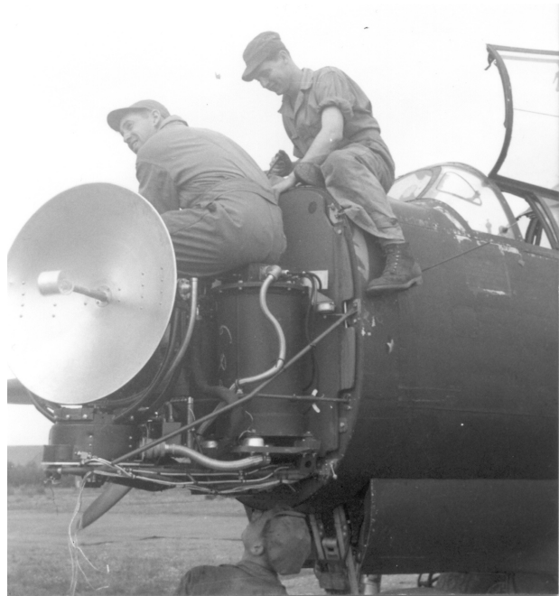
P-61 Radar repairs, Bolinski & Fields on top of plane, Rich Ziebart below radar while at Fritzlar, Germany.
